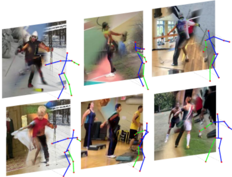
Figure 3. Given a candidate 3D pose, our algorithm selects for each joint an image whose annotated 2D pose locally matches the projected 3D pose. The selected images are then combined to generate a new synthetic image by stitching local image patches in a kinematically constrained manner. We show 6 examples corresponding to the same 3D pose observed from 6 different camera viewpoints.
