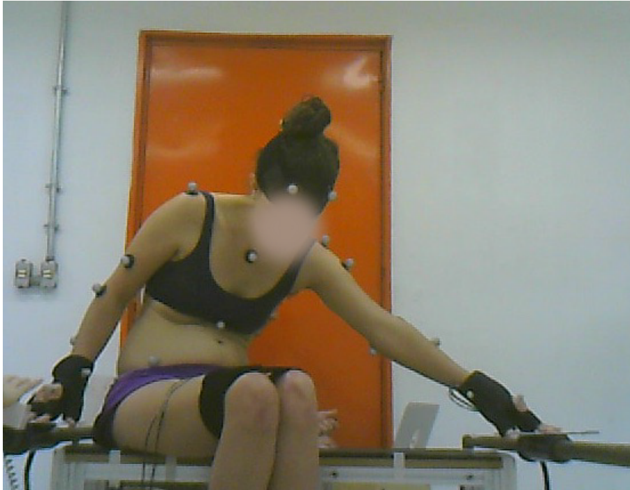
Figure 16. Experimental set-up. The gloves embed pressure sensors. It is possible to see the markers over the subject body, which are captured by the motion capture system.
