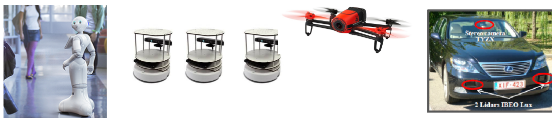
Figure 5. Most of the Chroma platforms: the Pepper robot, a fleet of (22) Turtlebot 2, one of the 4 Bebop drones and the equipped Toyota Lexus.
