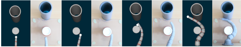
Figure 2. Top: Real cable-driven soft robot, Bottom: Corresponding motion computed by the simulated inverse model. The input of the inverse model is the motion of the robot's tip.
