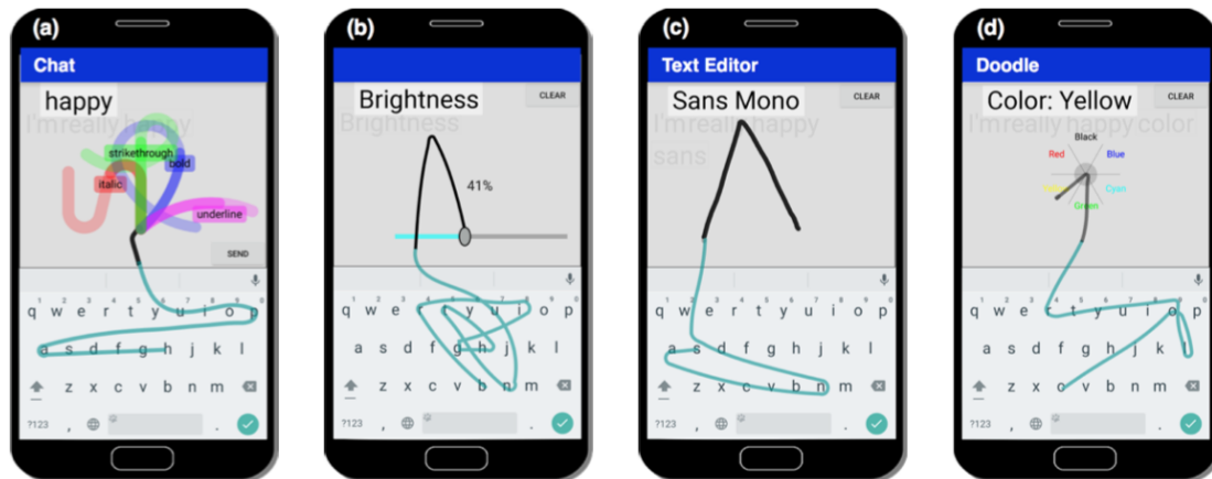
Figure 3. CommandBoard creates a new command gesture input space above a soft keyboard. Users can: a) type 'happy' and use a dynamic guide to style it as bold; b) type 'brightn', draw an execute gesture and adjust the brightness slider; c) type 'sans', choose 'sans mono' and draw an execute gesture to change the font; d) type 'color', select yellow in the marking menu to change the brush color.
