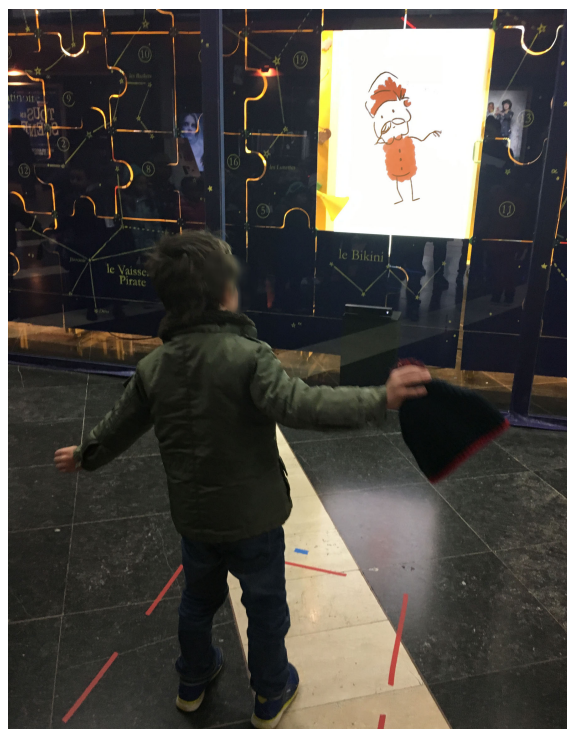
Figure 4. The interactive Christmas window: the Santa character mimics the movements of the user in front of the window, but also uses reinforcement feedback to shape the movements of the user.
