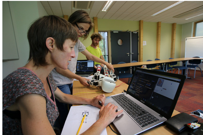
Figure 6. Using Snap! to program a robot by demonstration and create complex choreographies
