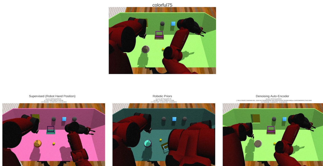
Figure 19. Nearest neighbors retrieved in the learned state space. The neighbors should represent the same button-hand relative position. Performance is shown in a left-right decreasing performance for the supervised (hand position) learning, 5 robotic priors and the autoencoder (better seen in video material)
