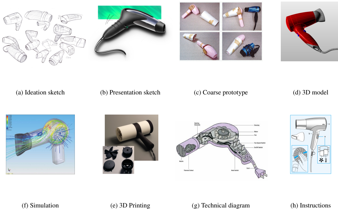
Figure 2. Various representations of a hair dryer at different stages of the design process. Image source, in order: c-maeng on deviantart.com, shauntur on deviantart.com, "Prototyping and Modelmaking for Product Design" Hallgrímsson, B., Laurence King Publishers, 2012, samsher511 on turbosquid.com, my.solidworks.com, weilung tseng on cargocollective.com, howstuffworks.com, u-manual.com
