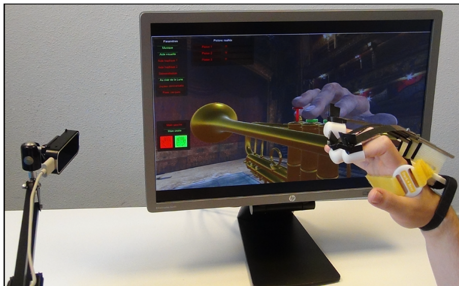
Figure 8. The FlexiFingers is a multi-finger device, combined with a pseudo-haptic approach, that can be used in music learning applications for instance.
