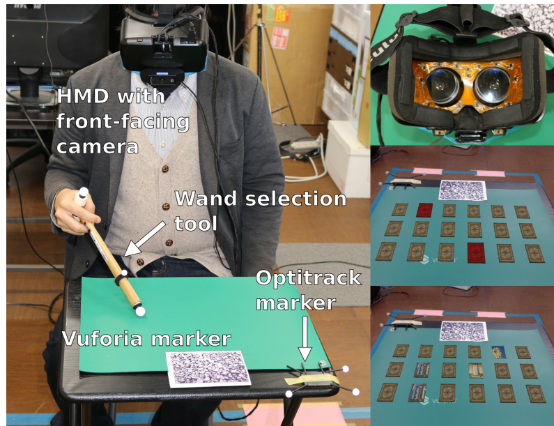
Figure 10. A participant wearing the Expression-Wear and playing our AR memory card game. Top right: The ExpressionWear embedded in the Oculus Rift. Middle and Bottom right: two states of our AR memory card game.
