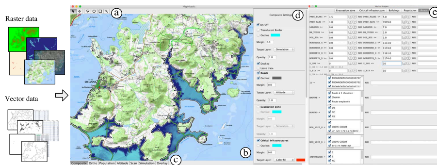
Figure 6. A proof-of-concept implementation of the MapMosaic dynamic compositing model and interaction techniques. (a) Toolbar to navigate the map, and to create & select areas. (b) Map viewer. (c) Access to individual layers. (d) Compositing area inspector. (e) Query builder for compositing region filters.
