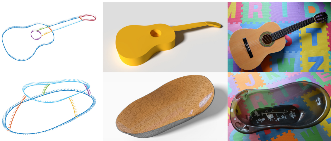
Figure 9. Shape from sensors: Curve networks on surfaces from 3D orientations. Guitar and bathtub scanned using the Morphorider. Left to right, reconstructed networks, surfaces computed from the networks, the scanned objects. The guitar shape was created by extruding the surfaced network.
