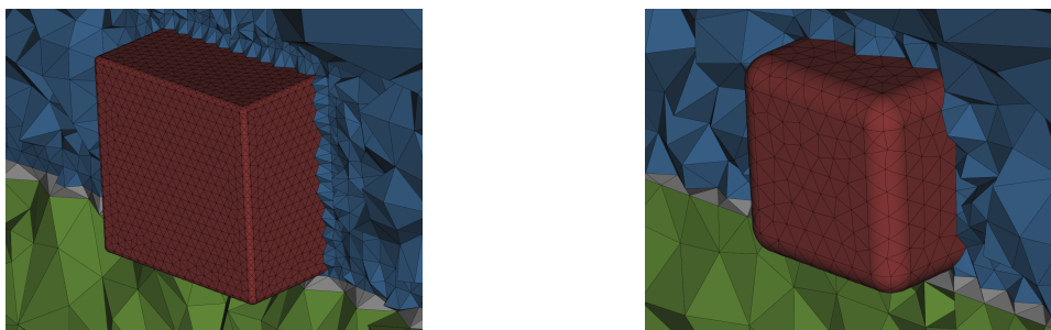
Figure 9. Meshes of rounded nanocubes with rounding radii ranging from 2 to 10 nm. Red cells correspond to the cube. The latter lies on the dielectric spacer (gray cells) and the metallic plate (green). Blue cells represent the air surrounding the device.
