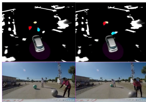
Figure 5. Image from the Velocity Display module : in every occupied cell of the grid, the average velocity is represented by a color code, the hue being based on the orientation, the saturation on its norm. A static cell is white, a cell moving in the same direction as the vehicle is red, in the opposite direction in blue. In the grid can be seen the moving balloons, the pedestrians being static.
