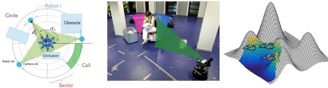
Figure 11. (a) Concentric navigation model and (b) its experimental setup. (c) Illustration of the local search method for multi-UAV coverage.
