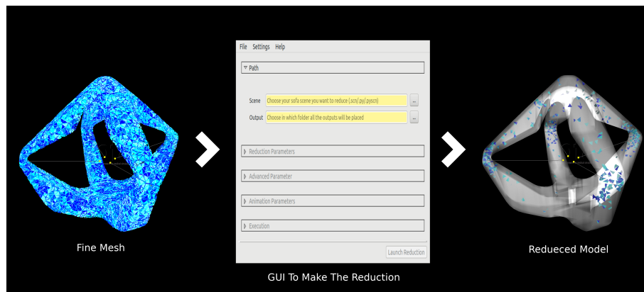
Figure 3. From a computationally intensive simulation to a surrogate version saving accuracy
