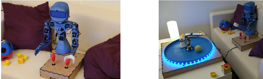
Figure 17. Robotic setup. Left: a Poppy Torso robot (the learning agent) is mounted in front of two joysticks. Right: full setup: a Poppy Ergo robot (seen as a robotic toy) is controlled by the right joystick and can hit a tennis ball in the arena which changes some lights and sounds.
