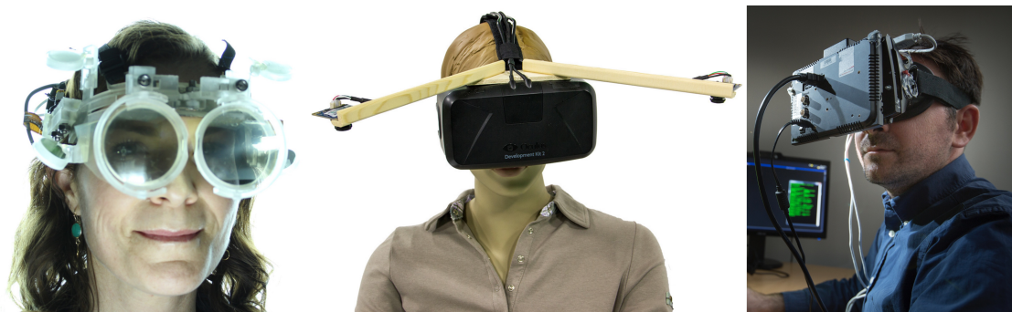
Figure 12. We presented novel display technologies, including but not limited to (left-to-right) varifocal augmented reality displays, body-tracking displays and focus-tunable displays.
