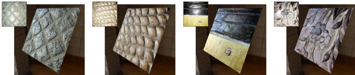
Figure 6. From a single flash photograph of a material sample (insets), our deep learning approach predicts a spatially-varying BRDF. See supplemental materials for animations with a moving light.
