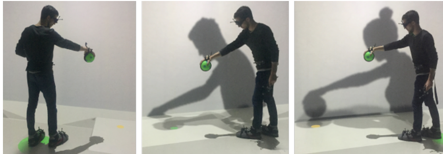
Figure 5. Various virtual shadows conditions. The participants performed a positioning task with 3 different virtual shadow conditions: None (N) (left), Male (M) (middle), Female (F) (right). The real shadow of the user is visible on the floor but does not match the natural behavior of a shadow in the virtual environment and is not taken into consideration.
