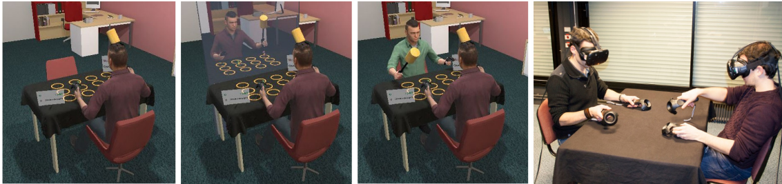
Figure 3. Studying the sense of embodiment in VR shared experiences: Setup of the experiment. Each user was able to interact in the virtual environment with his own avatar, while the physical setup provided both a reference frame and passive haptic feedback. From left to right: experimental conditions Alone, Mirror and Shared; Physical setup of the experiment.
