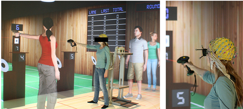
Figure 19. Experimental setup used in our sport performance study. (Left) Subjects were standing in our immersive projection system and were able to interact with the system using an ART Flystick. (Right) Subjects were wearing a high-density 64 channels EEG cap.
