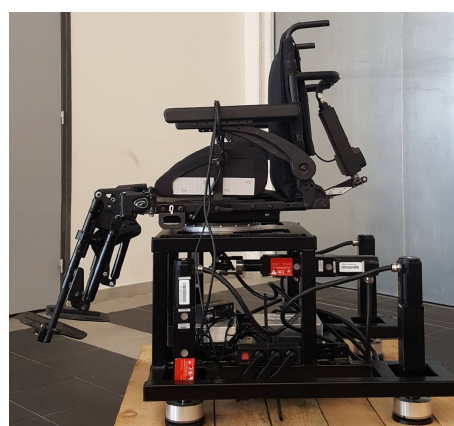
Figure 2. Upgrade of the Immersia platform: two new devices installed. (Left) "Scale-One" Haptic system for one or two users. (Right) Motion platform for powered wheelchair simulation.
