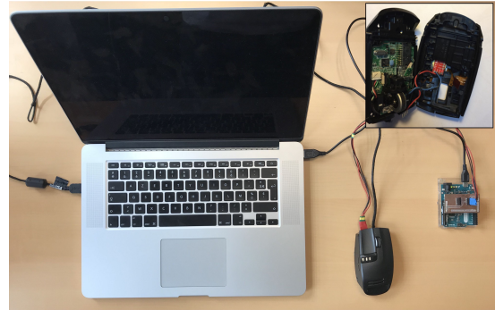
Figure 2. (left) General description of our real-time input prediction method, with step numbers. Input in green, previously computed variables in blue, general parameters in yellow, optimized parameters in orange. (right) Our hybrid setup for input prediction comprises a Logitech G9 Laser Mouse connected via USB to the host computer with the MPU-9250 chip embedded inside, which is itself connected to an Arduino board.
