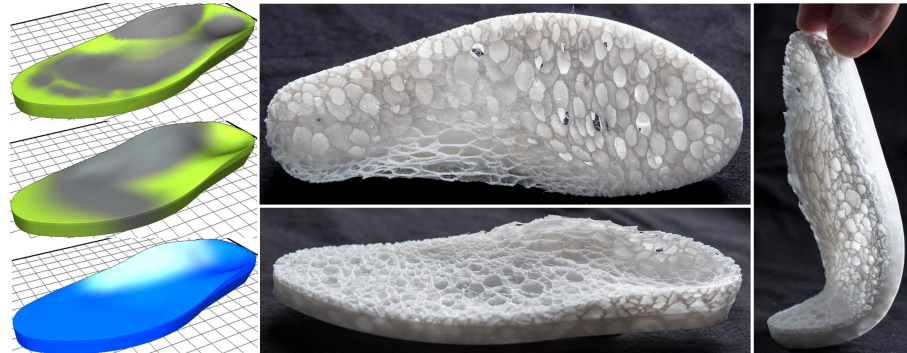
Figure 3. A 3D printed shoe sole. Left: Control fields used on the model, density (top), orthotropy strength (middle) and angle (bottom). Right: Printed shoe, top, side and bending. The shoe is printed without any skin to reveal the foam structure.
