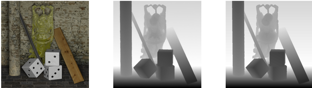
Figure 2. Estimated depth map (middle) for the light field 'Buddha' in comparison with the ground truth (right).
