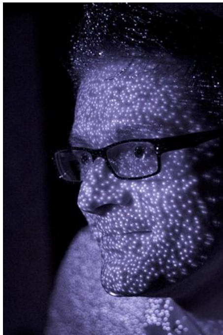
Figure 14. Structured light. A calibrated camera and projector (typically both near infrared) are placed at a fixed, known baseline. The structured light pattern helps establish correspondence between observed and projected pixels. Depth is derived for each corresponding pixel through triangulation. The process is akin to two stereo cameras, but with the projector system replacing the second camera, and aiding the correspondence problem.
