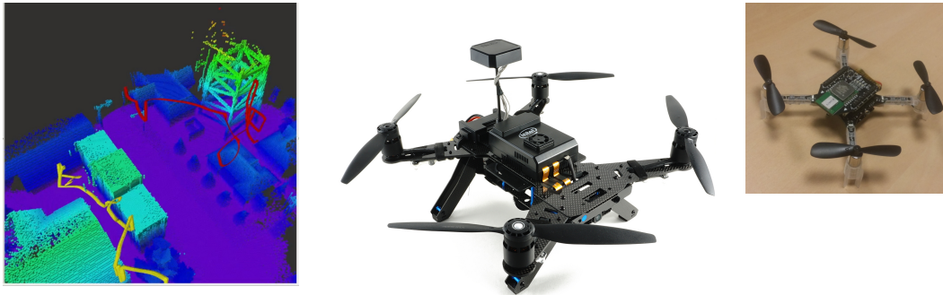
Figure 21. (a) UAVs Chroma simulator (b) Intel Aero quadrotors platform (c) Crazyflie micro-UAV platform extended with UWB decawave chip.
