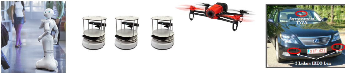
Figure 4. Most of the Chroma platforms: the Pepper robot, a fleet of (22) Turtlebot 2, one of the 4 Bebop drones and the equipped Toyota Lexus.
