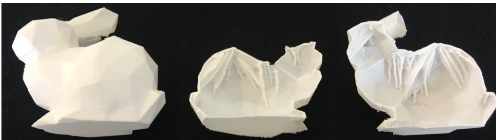
Figure 4. A 3D bunny model printed with our internal ribbed supports. It is mostly empty, with the ribbed vaults providing just enough support to prevent filament to fall during manufacturing.
