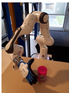
Figure 5. Rainbow advanced manipulation platform. a) One of the two Panda lightweight arms from Franka Emika, with mounted the Pisa SoftHand, b) the Reflex TakkTile 2 gripper that could be mounted on the Panda robot end-effector.
