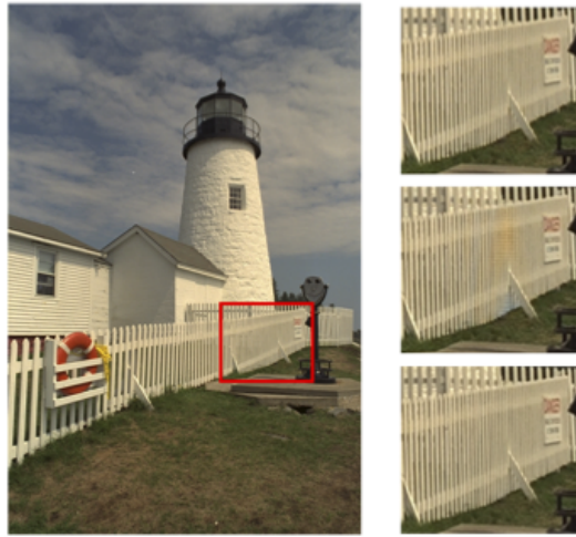
Figure 9. Demosaicking result obtained by our method. Top right: Ground truth. Middle: Image demosaicked with our sparse coding baseline without non-local prior. Bottom: demosaicking with sparse coding and non-local prior. The reconstruction does not exhibit any artefact on this image which is notoriously difficult for demosaicking.
