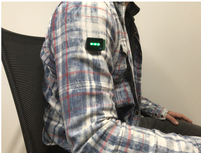
Figure 11: Sensor positioning for initial shoulder movement data collection.
