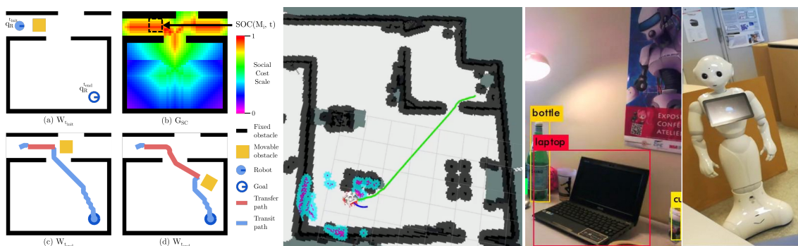
Figure 14: (a) S-NAMO planning illustration (b) Pepper's navigation and mapping (c) Object detection with Pepper based on vision/deep learning techniques.
