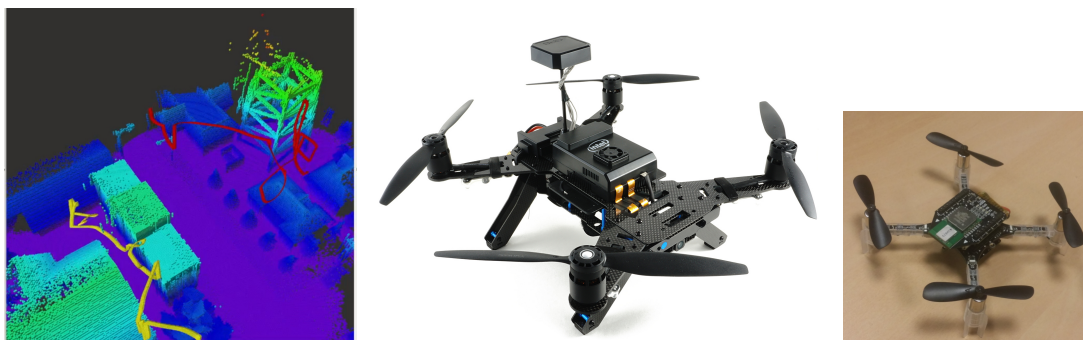
Figure 15: (a) UAVs Chroma simulator (b) Intel Aero quadrotors platform (c) Crazyflie micro-UAV platform extended with UWB decawave chip.
