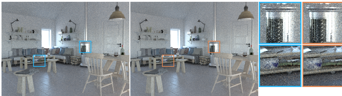
Figure 12: Equal-time comparisons (2 minutes). Our method (right, orange) reduces noise compared to prior work by efficiently guiding paths based on the product of the BSDF and incoming radiance at each path vertex.
