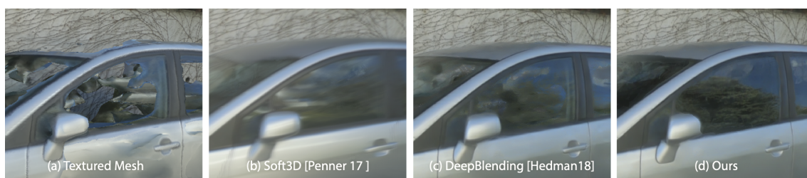
Figure 9: We propose a new solution for rendering captured cars, and in particular their reflective, semi-transparent windows. A textured mesh from multi-view stereo reconstruction (a) is missing the window geometry. Recent free-viewpoint Image-Based Rendering algorithms (b, c) are not designed to handle the rendering of both the reflection of blue sky, green leaves and the transmissive content (car interior). Our method (d) handles this by computing real-time reflection flows on an ellipsoid approximation of the curved window surface, based on our estimate of a smooth hull of the car that exploit semantic labels in the input images.
