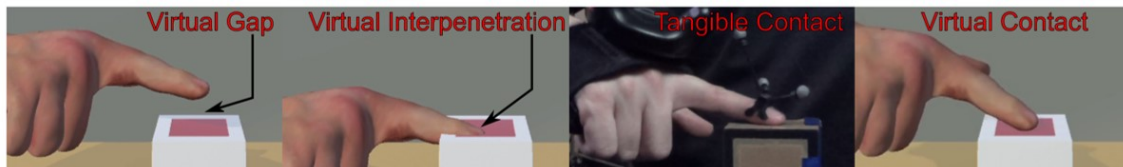
Figure 17: Using capacitive sensing to reach a better visuo-haptic synchronization upon contact and preserve immersion during interaction in VR.
