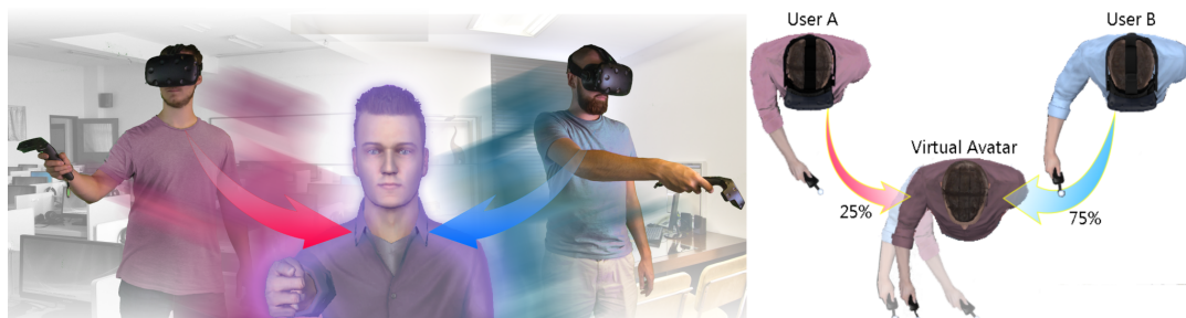
Figure 10: Our “Virtual Co-Embodimen” experience enables a pair of users to be embodied simultaneously in the same virtual avatar (Left). The positions and orientations of the two users are applied to the virtual body of the avatar based on a weighted average, e.g., “User A” with 25% control and “User B” with 75% control over the virtual body (Right).
