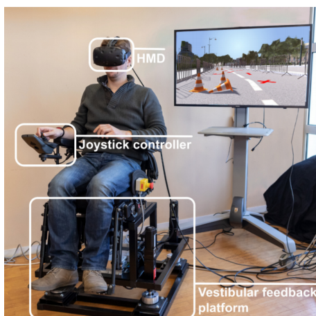
Figure 6: VR simulator for wheelchair driving with vestibular feedback.
