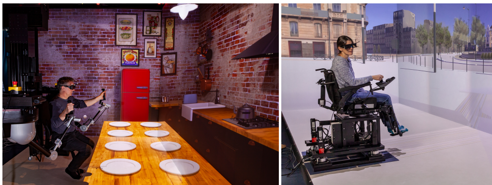
Figure 2: Immersia platform: (Left) “Scale-One” Haptic system for one or two users. (Right) Motion platform for a powered wheelchair simulation.
