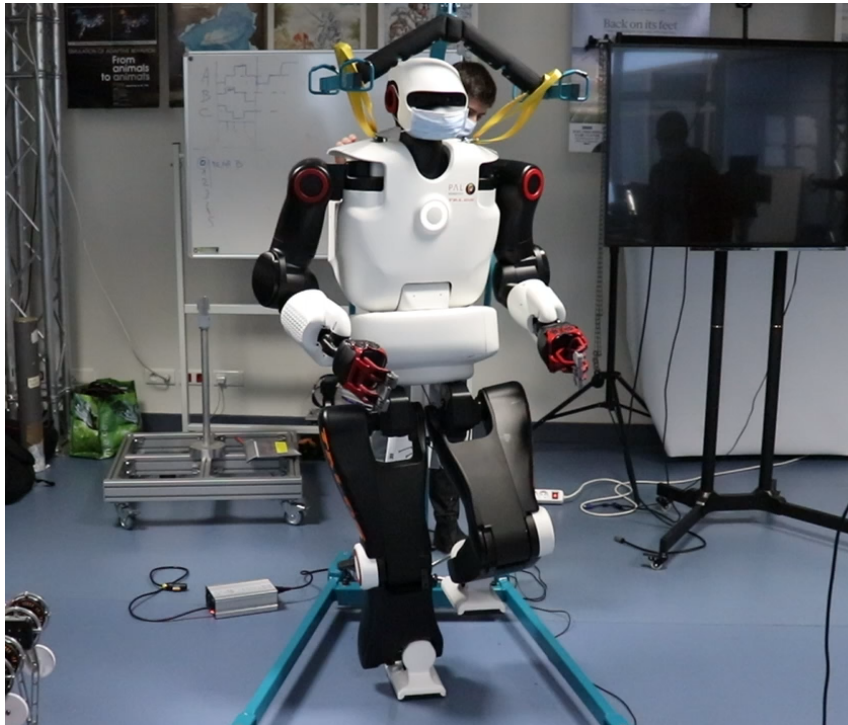
Figure 1: Talos on one foot, running our whole-body controller. At 1000 Hz, the robot uses a quadratic programming solver to compute the position of the 32 joints so that the feet and the hands are at the right position while (1) ensuring that the center of mass stays on top of the center of the foot, (2) there is no self-collision, (3) all the joint limits, velocity limits, and acceleration limits are respected. The ZMP (Zero Moment Point) stabilizer uses the force-torque sensor of the ankle to reject external perturbations.
