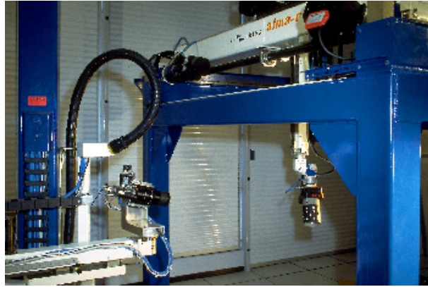
Figure 2: Rainbow robotics platform for vision-based manipulation
