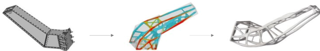
Figure 9: Antenna bracket. Advances in topological optimization and additive manufacturing yield increasingly complex shapes with reduced weight. Left: original design. Middle: topological optimization. Right: new design.
