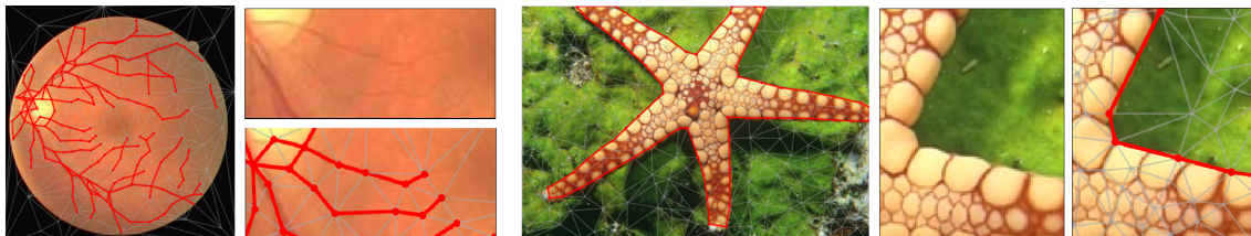
Figure 2: Example applications of Delaunay Point Processes to extract planar graphs representing blood vessels in retina images (left), and complex polygons representing object silhouettes (right). The point distribution creates a dynamic Delaunay triangulation while edge and facet labels specify the geometric structure (see red edges on close-ups).
