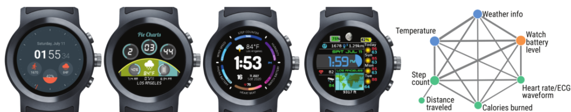
Figure 10: Visualizations for Smartwatches with increasing complexity. On the right, visualization of study results that show which types of information are commonly displayed on watchfaces.
