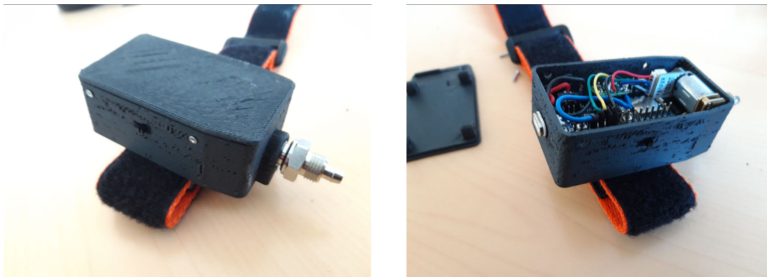
Figure 17: Example of mechanical module including power storage, actuation and control unit with bluetooth communication
