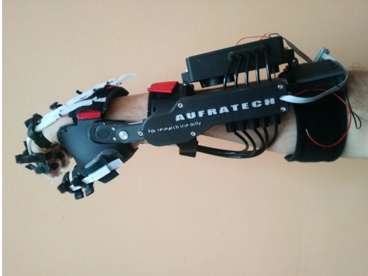
Figure 15: Aufratech orthosis and a pod from Vivaltis Phoenix stimulator (two channels)
