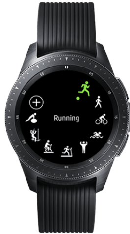
Figure 5: Smartwatch Samsung Galaxy used for long duration recordings of wrist movement by acquisition of accelerometer data from Parkinson tremors, autonomously starting and stopping at predefined hours of the day.
