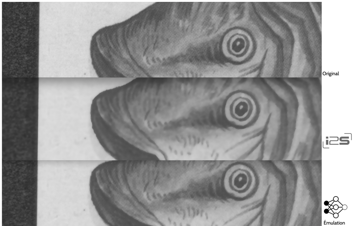
Figure 3: Top: Original image. Center: Denoised using i2s method. Down: Emulation. Higher image quality can be obtained by using an emulation approach which provide an image quality compared to that of an iterative algorithm.
