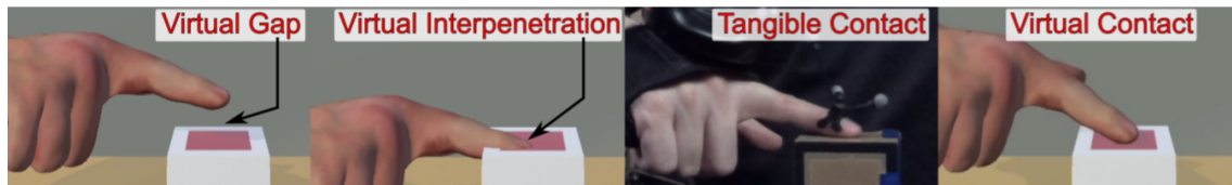
Figure 16: Representative issues while using standard optical tracking systems (left) vs. our integrated capacitive-based approach (right). By combining tracking information from standard optical tracking systems with proximity information from a capacitive sensor, we are able to re-target the virtual fingertip toward the virtual surface, achieving a better synchronization between tangible and virtual contacts.
