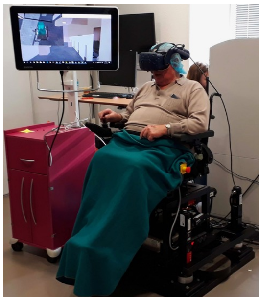
Figure 5: Virtual Reality condition setup of our clinical study with our power wheelchair simulator.
