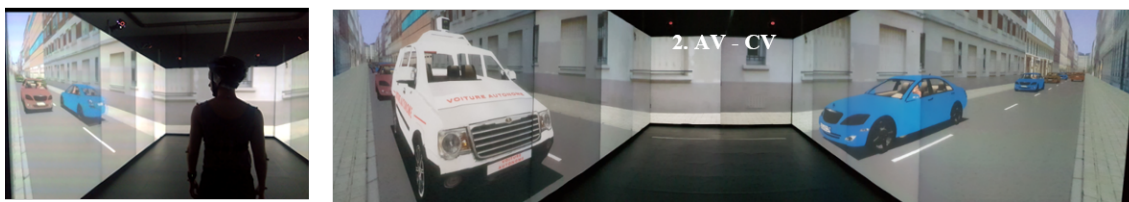
Figure 19: Illustration of the experiment in the simulator room to study the interaction between a pedestrian and self-driving and conventional cars.
