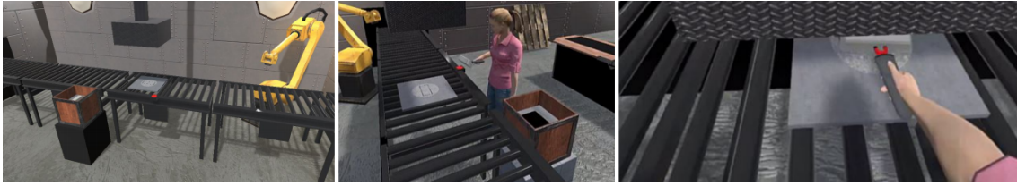
Figure 12: Overview of the virtual environment representing a factory (left), an avatar representing a user placing an ingot on the plate arrived on the conveyor lay (center) and the crusher threatening the user by suddenly going down while the user's hand is under it.
