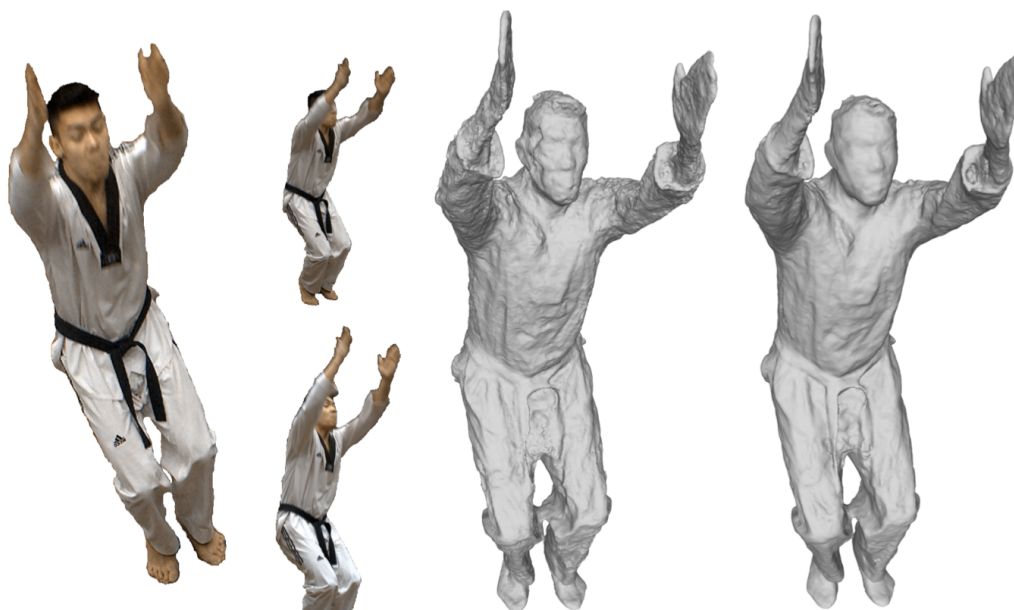
Figure 2: (Left) 3 input images, (middle) plane based classifier, (right) volumetric classifier. The face is highly occluded in many views (left) making the reconstruction noisy and inaccurate when using a planar support whereas the volume counterpart yields smoother and more accurate details.
