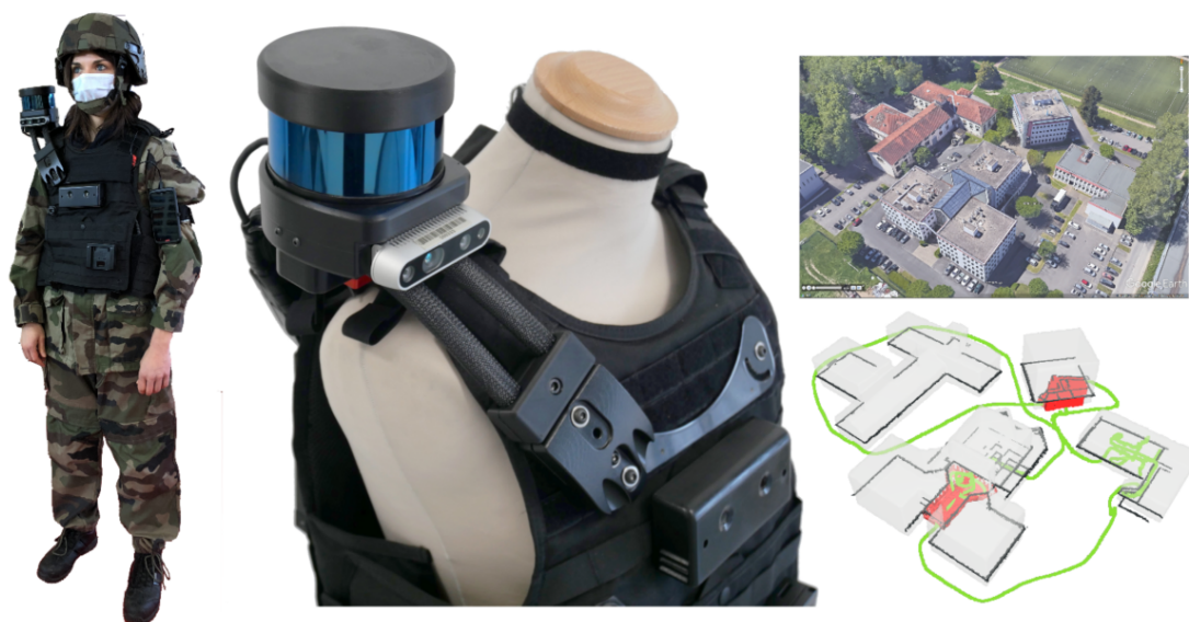
Figure 7: WeCo-SLAM system. The group of LVI sensors is mounted on the shoulder of a tactical waistcoat. This allows its wearability by a trained agent that performs recon missions under challenging conditions. Example results are shown right, where the followed trajectory is shown in green and the outdoor/indoor reconstruction of visited buildings is shown in gray and red, respectively. Predicted GPS coordinates are sent via radio to a ground station that monitors the agent's position in real-time.
