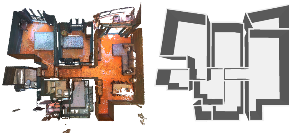
Figure 8: Floorplan generation. Left: the algorithm departs from raw point clouds as input data. Right: the floorplan of the indoor scene is reconstructed as a planar graph where each simple cycle represents the polygonal boundary of a room. Note that the 2D floorplan is converted into a 3D CAD model for visualization purposes.
