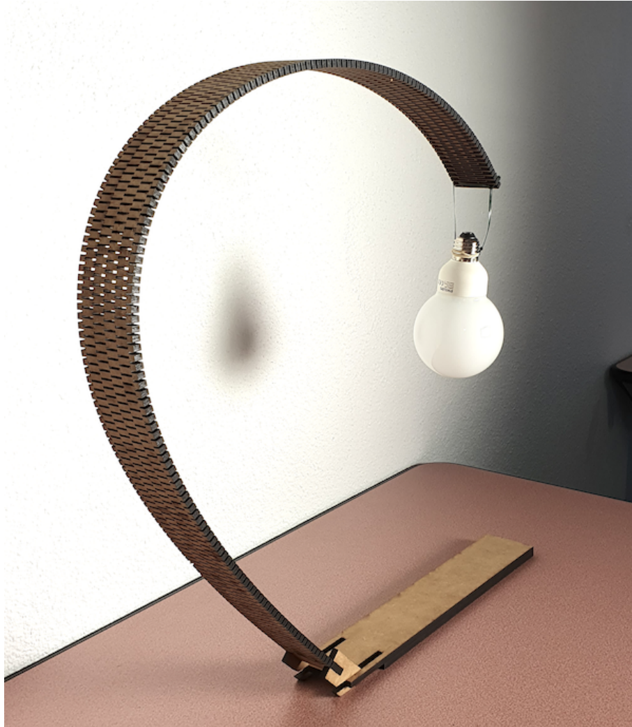
Figure 3: Laser-cut bending-active structure whose silhouette matches an input target curve provided by the user. Under the hood, our algorithm optimizes the stiffness profile of the bending-active structure and automatically converts it into cutting patterns of optimal sizes.
