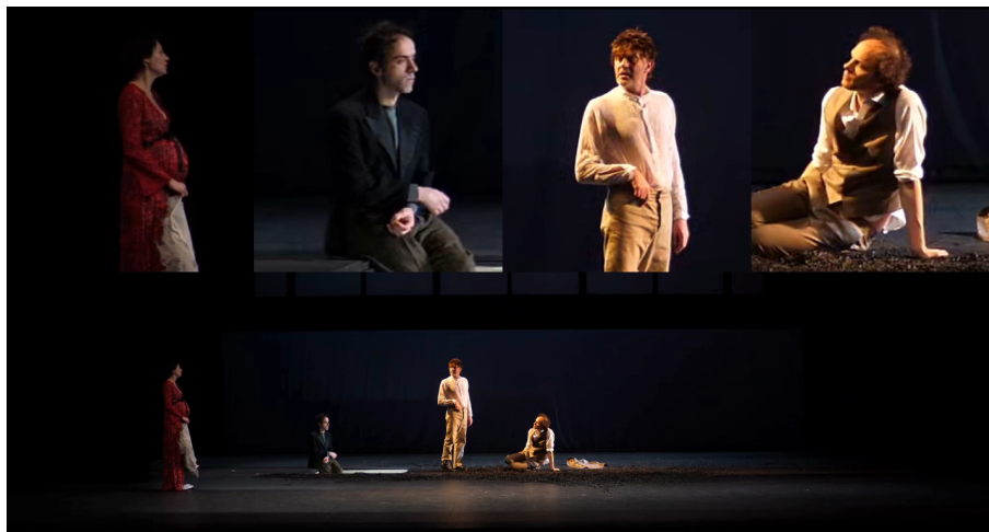
Figure 7: KinoAI workflow. Bottom: The stage is filmed with a fixed camera in ultra-high definition. Top: We generate candidate shots with different compositions on the server side and allow remote users to edit them into movies on the client side.
