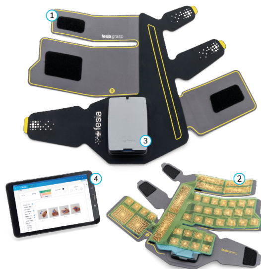
Figure 9: Fesica Grasp upper limb rehabilitation stimulator. (1) Protective garment (2) Hydrogel surface electrode matrix (3) Electrical Stimulator (4) Parametrization tablet for clinicians
