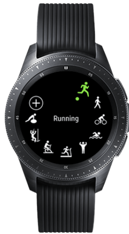
Figure 20: Smartwatch Samsung Galaxy used for long duration recordings of wrist movement by acquisition of accelerometer data from Parkinson tremors, autonomously starting and stopping at predefined hours of the day.
