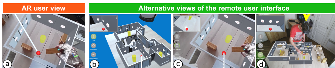
Figure 3: A user wearing an AR headset and a remote desktop collaborator perform a physical furniture arrangement task around a virtual 3D house model. (a) AR user’s view displayed in the headset and three alternative views of the remote collaborators available in our user interface: (b) a fully virtual view, (c) a first-person view streamed from the headset, and (d) an external view streamed from a depth camera.
