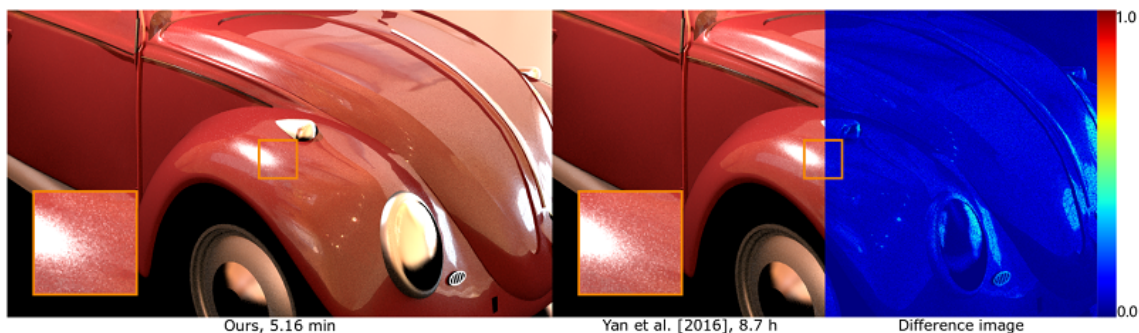
Figure 8: Comparison between our method and Yan et al. [2016] on the Car scene, using a seamlessly tileable normal map of metallic flakes with resolution 2K \times 2K under geometric optics. The rendered glints are almost identical, but our method costs less than 1 % of time compared to Yan et al. [2016], and does not scale with the view distance.
