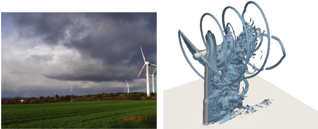
Figure 2: Aerogust project. Left: met mast after its installation. Right: flow around a NREL wind turbine rotor (as predicted by NaSCar).
