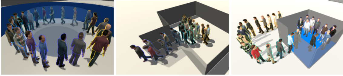
Figure 12: Snapshot of crowd motions generated using the one-man-crowd approach. A single user successively embodies each displayed virtual agent in the order indicated by the highlighting colour (from blue to yellow). We studied 3 scenarios that replicated existing experiments from left to right: circular unidirectional flow, bottleneck situation, inflow behaviour (entering a lift).
