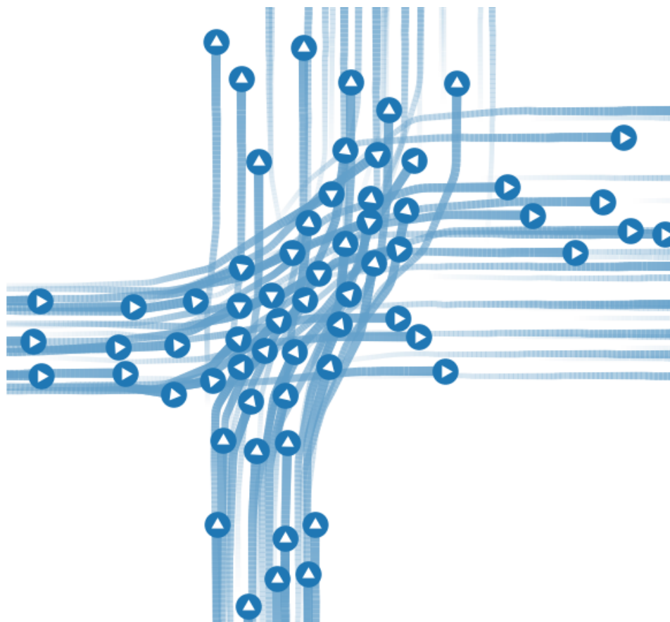
Figure 7: Simulation of two agent flows crossing at 90^\circ using three different motion strategies, and their respective score S_{QF} according to a quality function (a) Agents are steered using the Power Law model (PL, blue). Note that some agents are dragged along a diagonal towards the up-right direction, hence deviating them from their goal. PL ( S_{QF} = 67 )
