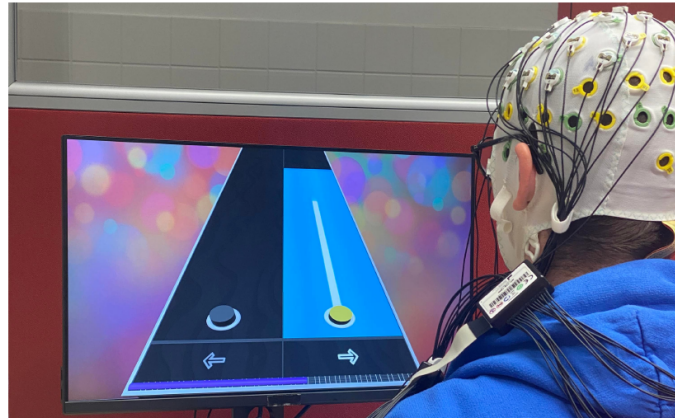
Figure 3: The new visual feedback and gaming environment of the Brain Hero mental imagery-based BCI training, during actual use.
