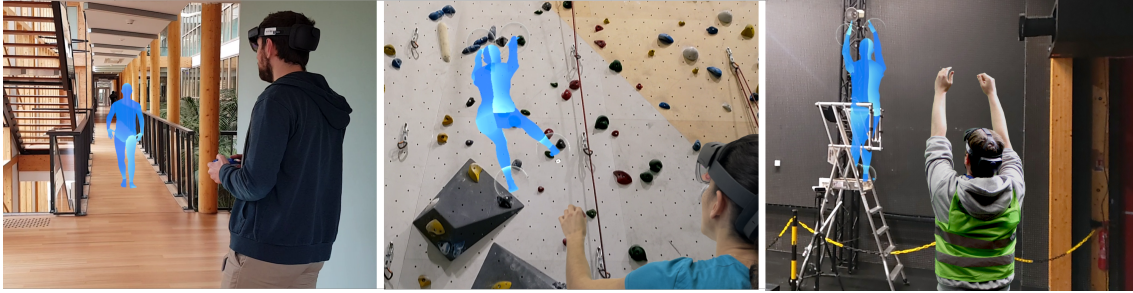
Figure 4: Control of self-avatars visualized through an Augmented Reality headset to better perceive interactions and affordances in the physical surroundings. Left: Testing fire exit paths with a gamepad. Center: Planning and testing a route before climbing by controlling the avatar's limbs with gestures. Right: Evaluating possible actions on a distant step stool with body-tracking mapping.
