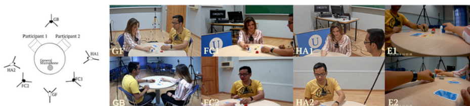
Figure 12: Recording environment (we use FC view for our work). Six tripod-mounted cameras, namely GB: General Back camera, GF: General Frontal camera, HA: individual High Angle cameras and FC: individual Frontal Cameras, and two ego cameras E (one per participant, placed around their neck). From left, Position of cameras, general microphone and participants and example of the time-synchronized 8 views.
