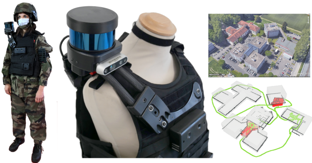
Figure 8: WeCo-SLAM system. The group of LVI sensors is mounted on the shoulder of a tactical waistcoat. This allows its wearability by a trained agent that performs recon missions under challenging conditions. Example results are shown right, where the followed trajectory is shown in green and the outdoor/indoor reconstruction of visited buildings is shown in gray and red, respectively. Predicted GPS coordinates are sent via radio to a ground station that monitors the agent's position in real-time.
