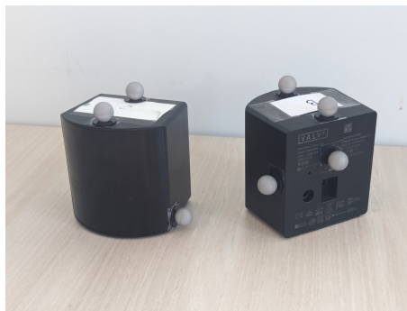
Figure 8: Visually tracked Lighthouse v2 basestation
