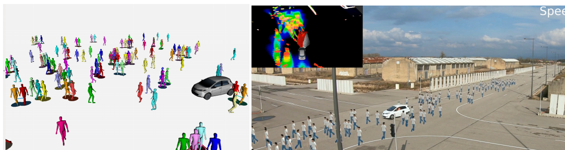
Figure 4: a. Illustration of a typical scene of an AV sharing its space with pedestrians. b. Illustration of a zoe navigate a simulated crowd using augmented reality.
