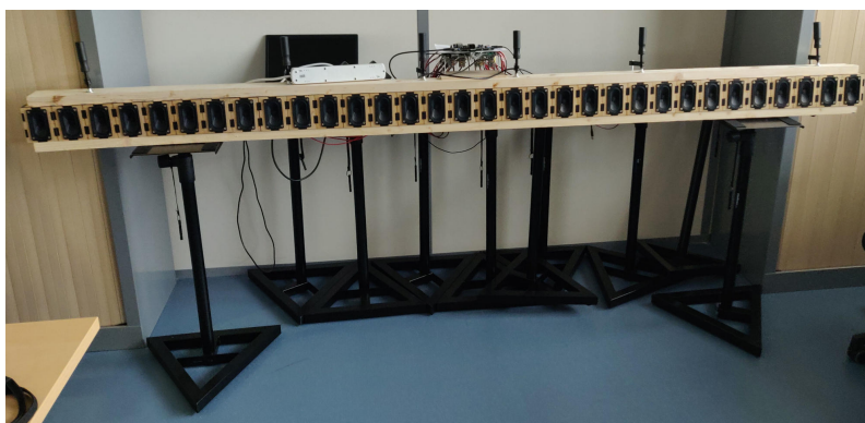
Figure 9: The Wave Field Synthesis system developed as part of PLASMA.
